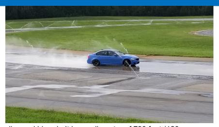
complex is the B2 skid pad, which is no ordinary skid pad. It has a diameter of 790 feet (120 m radius), giving it almost a half mile circumference. It is made of polished concrete and it is slicker than greased ice when wet.
